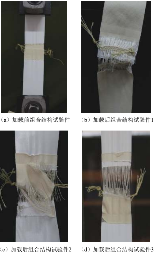
图 11 缝绉与热合组合形式试件强度试验现象 Fig. 11 The strength test of sewing and thermal combination specimens
