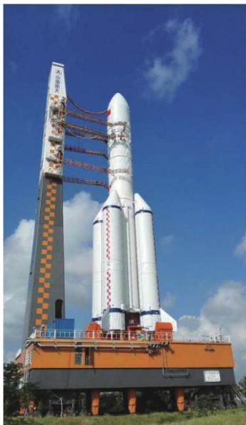
图9 “长征五号”运载火箭垂直转运 Fig. 9 Vertical transportation of LM-5
