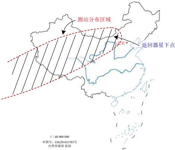
图 5 对返回器可见的测站区域 Fig. 5 The ground station visible region for reentry module
