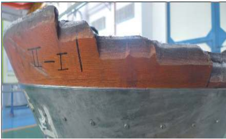
图2 喷管断口部位概貌 Fig. 2 General picture on fracture site of nozzle
