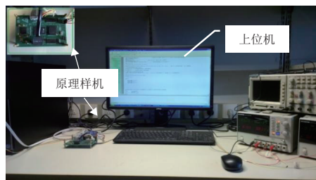
图 7 X射线脉冲星导航半物理仿真系统 Fig. 7 The semi-physical simulation system of the X-ray pulsar navigation
