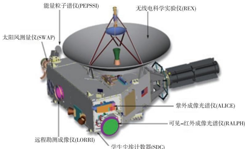
图 2 “新视野号”探测器携带的有效载荷<sup>[4]</sup>Fig. 2 The scientific instruments aboard on New Horizon space craft<sup>[4]</sup>
